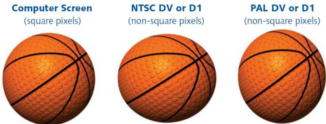
Figure 1: The pixel aspect ratio can produce undesirable image distortion if you do not compensate for the difference between square and non-square pixels.
