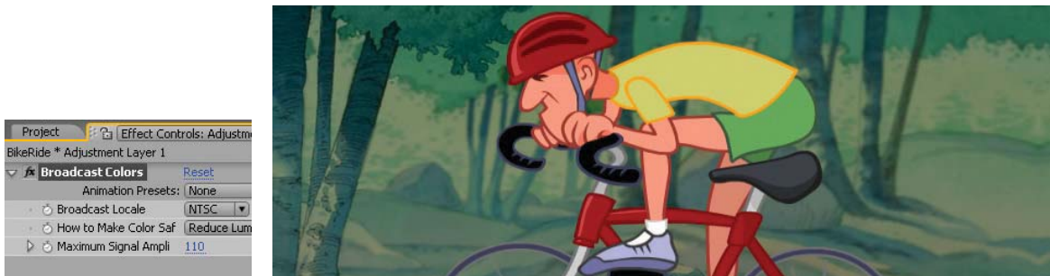
Figure 2.20: Apply the Broadcast Colors effect to an adjustment layer to keep the composition's color space within the color range allowed for NTSC and PAL video.
