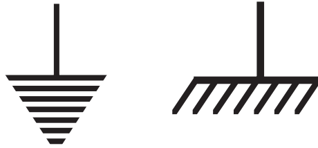
FIGURE 3.7 An icon like this indicates a grounding screw on equipment.
